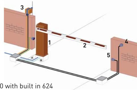
1. FAAC 620 with built in 624 BLD control board
